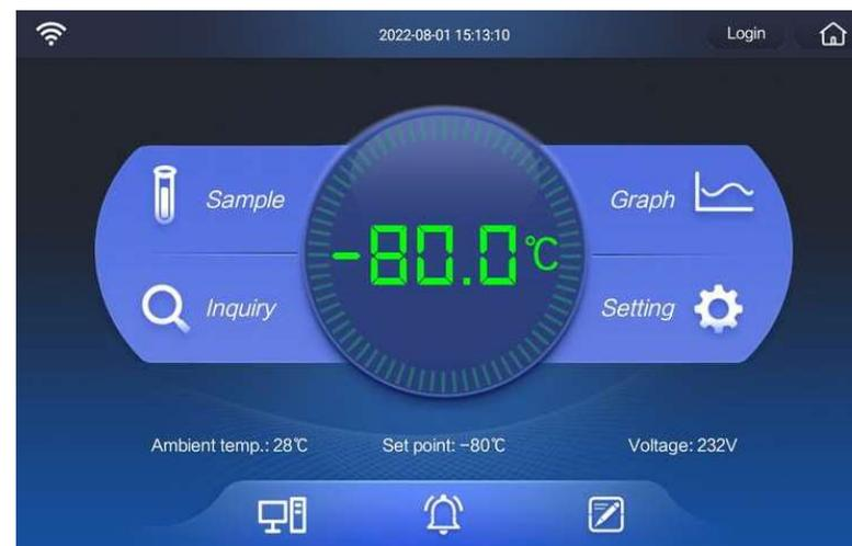
In the home page, it can display the real-time internal temperature, ambient temperature, set point, input voltage, backup system state (optional), network state, electromagnetic lock state (optional), user login status, freezer health status, temperature graph, and message/ note book, etc..
