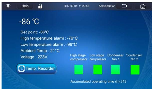
For the operation state of compressor / fan, "Green" indicates that it is running; "Grey" indicates that it is not running.
