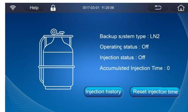
For the accumulated injection time, it displays the accumulated injection time since the last start-up.
