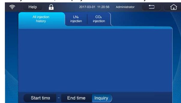
Enter/input "Start time-End time", and then click "Inquiry" to query the spraying record in this interval. One or several injection history can be deleted to the spraying history.
