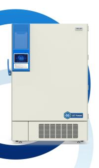
Cascade system ULT freezer that consists of two stages cascade cooling technology with absolute hydrocarbon refrigerant, which are R290 and R170 as natural gas. The inverter compressors programmed to help energy savings under long period preservation or provide fast temperature recovery while frequently door open to maintain specimens liveness.
